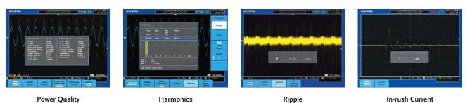
The Power Analysis software contains four measurement functions, including Power Quality, Harmonics, Ripple and Inrush Current. The Power Quality analysis function allows the measurements of Voltage, Current, Frequency, Power and other quality related parameters for power source efficiency improvement. The Harmonics analysis function performs evaluation of power waveform distortion and gives harmonic
