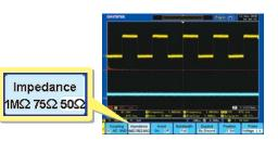
Three input impedance,  $1M\Omega$ ,  $75\Omega$ , and  $50\Omega$  are available for user's selection. The flexibility of impedance selections, including  $1M\Omega$  to get minimum loading effect,  $75\Omega$  to accommodate Video transmission applications and  $50\Omega$  to fit RF communication applications, extends the GDS-3000 Series utilization range.
